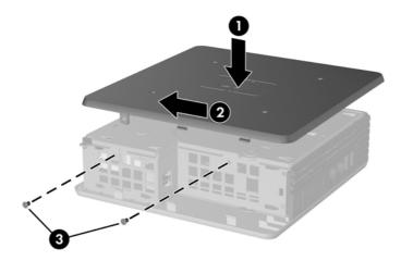
Figure 2-8 Replacing the side access panel
